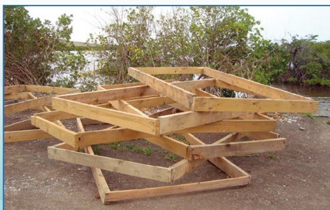
Figure 17 Example of racks. A capacity of approximately 100 plants per m 2 can make a good compromise. 1.6m x 6 m racks.
